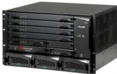
Figure 4: Multipoint Control Unit (MCU)
